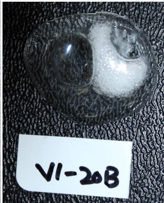
Photo 3. Representative photo of polymer liquid appearance after mixing and the resultant gel for the appearance description: Dissolved, foamy.
