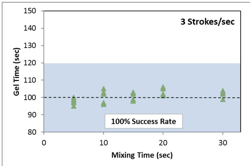
Figure 2. Probability of success at each mixing time for 1, 2 and 3 strokes/sec
