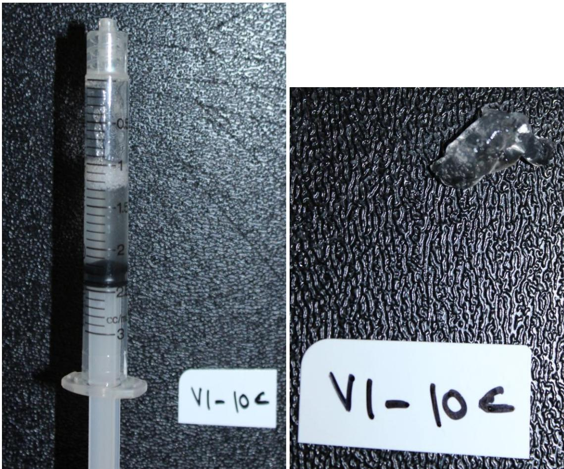
Photo 2. Representative photo of polymer liquid appearance after mixing and the resultant gel for the appearance description: Undissolved, foamy or partial foam.
